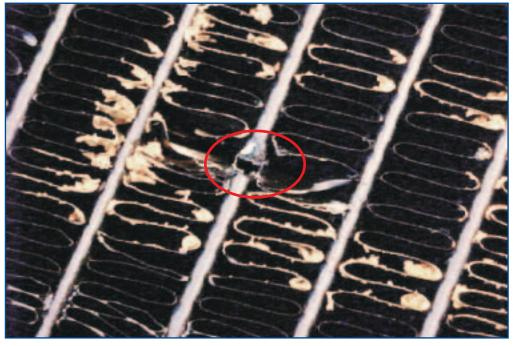
Punctured tube from rock or road debris
