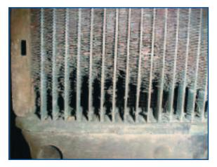
Illustration of Fin Deterioration
