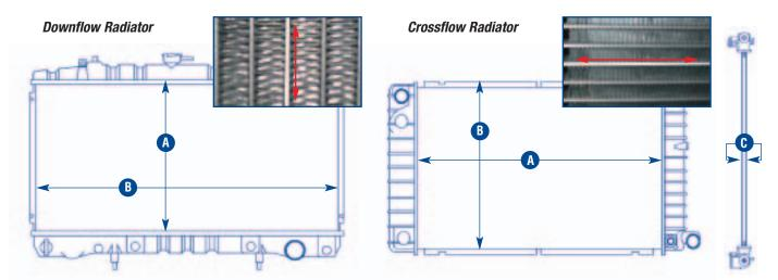
For both types of radiators: A = Height / B = Width / C = Core Thickness
