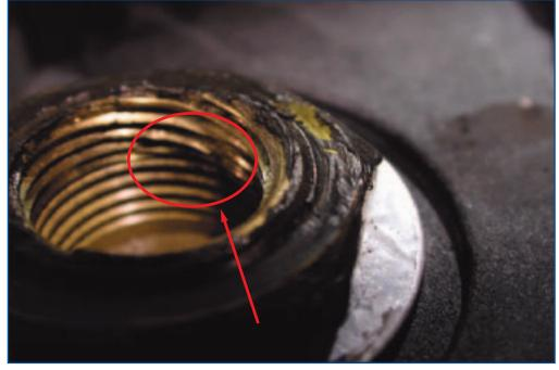
Stripped oil cooler threads
