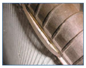
Blown Seam on a Plastic Aluminum Radiator
