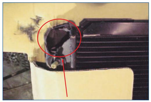
Damage due to shipping or handling
