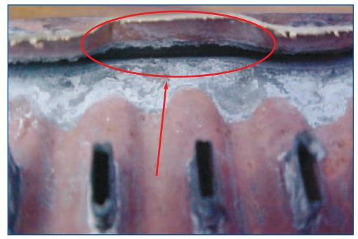
Premature seam failure
