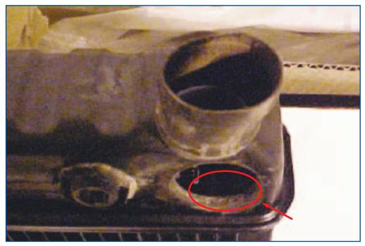
Loose or broken connection due to bad soldering
