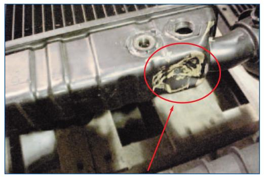
Damage due to shipping or handling
