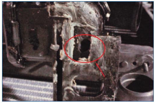
Drilled hole during installation
