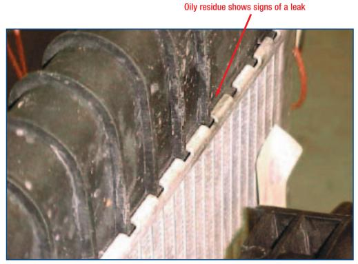
Tank Seam Leak due to a bad crimp or faulty gasket
