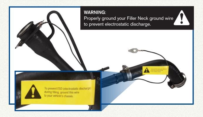
During the refuelling process, the friction created by fuel being introduced in the system may create static electricity which may cause ignition of the fuel.
