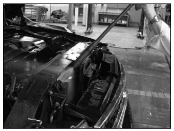
Watch for transmission oil coolers mounted directly onto a condenser. This is a favourite of transmission shops, but the transmission oil is 125C and the condenser is 60C. That means the transmis cooler heats up the condenser. That's the opposite of what a condenser does.
