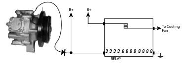
TO MAKE THE ELECTRIC FAN COME ON WITH COMPRESSOR, ADD A WIRE SPLICED FROM COMPRESSOR CLUTCH FEED TO HOT SIDE OF FAN RELAY COIL. SOLDER AND SHRINKWRAP A SIMPLE DIODE IN LINE SO THAT IF THE FAN COMES ON FROM THE RAD TEMP SENDER, IT WILL NOT TURN ON THE COMPRESSOR ALSO.
