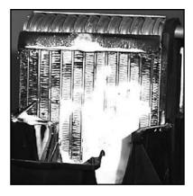
Some vehicles are equipped with an afterblow feature which keeps the blower motor on for a few minutes after the vehicle is shut down to dry out the evaporator case and prevent odours. Afterblow modules are also available as an add on for vehicles prone to odours. The seal at the end of the engine compartment must be in good shape and in proper position to prevent hot, smelly engine compartment air from getting into the inlet for the A/C system.
